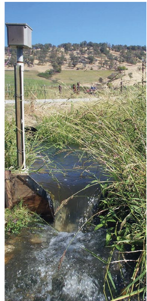
Top left, channelized runoff from the pasture was collected in a small basin. Above, V-weirs were fitted with, left, autosamplers to monitor E. coli concentrations.
